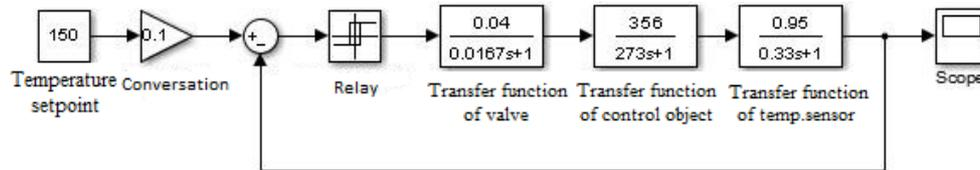
**Figure 3.1.** Simulink-model of the system for stabilizing the temperature during spraying
