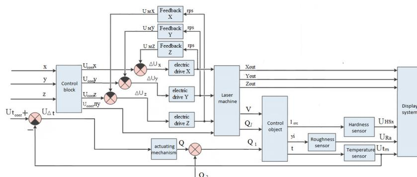
**Figure 1.** Structural diagram of the control system of the process of dioxide zirconium spraying and reflooding it with a laser beam onto the steam turbine blades.
