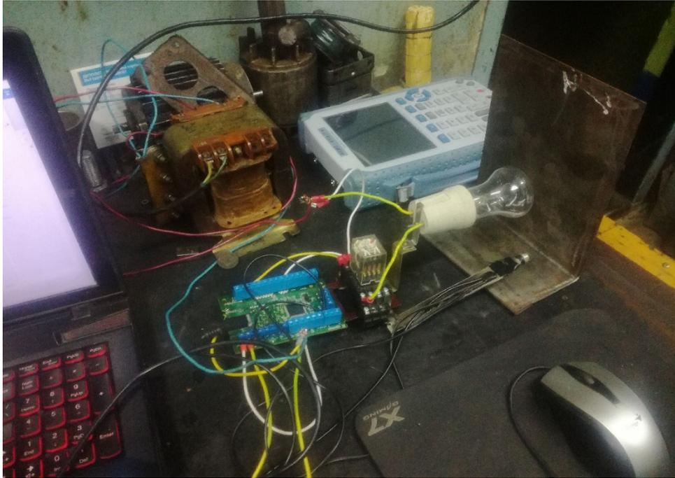
**Figure 4.2.** The stand of the temperature stabilization system
