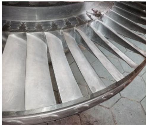
**Figure 2.** Rotor stage after application of zirconia.
