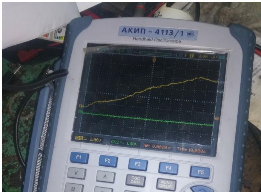
**Figure 4.3.** Changing the voltage at the output of the temperature sensor during the heating process
