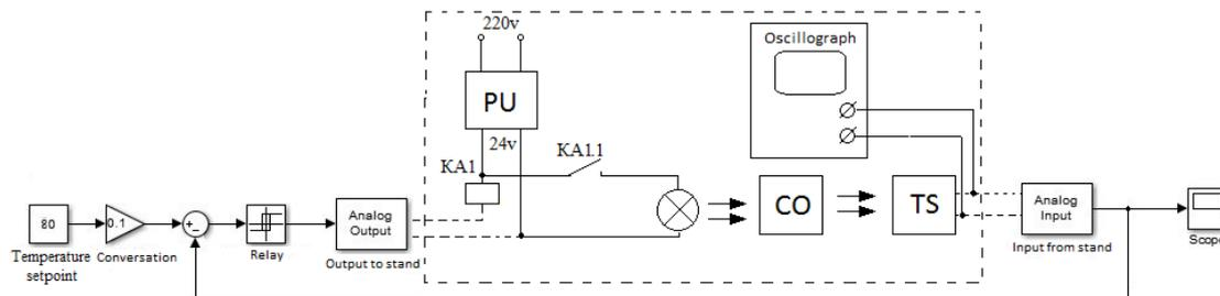
**Figure 4.1.** Simulink model with external devices connection
